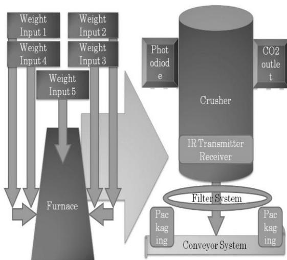
Fig. 1 A Basic Layout of the Complete Alloy Making Industrial Process.
