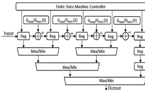
Fig 3.[1] Circuit Diagram Of The Dilation/Erosion Module For A Five-Point Operation
