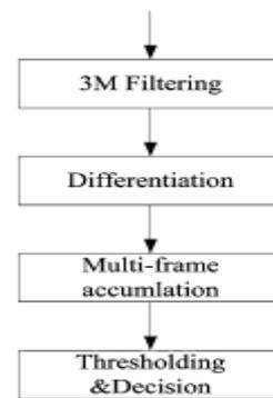
Fig. 2. Block Diagram of Proposed QRS Detection Algorithm
