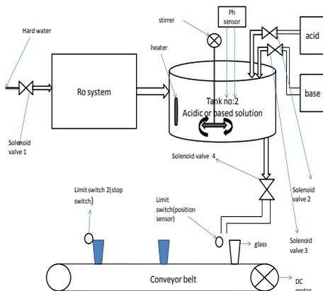
**Fig2. Basic Block Diagram of Water Treatment Plant**
