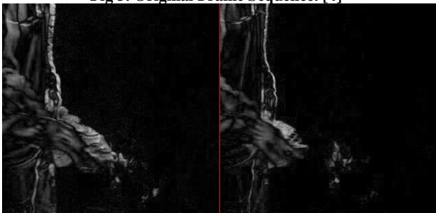
Fig 4. Motion Detected By Frame Differencing. [4]
