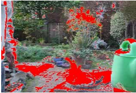
Fig 7. Fire-Color Classification sans Motion Detection
