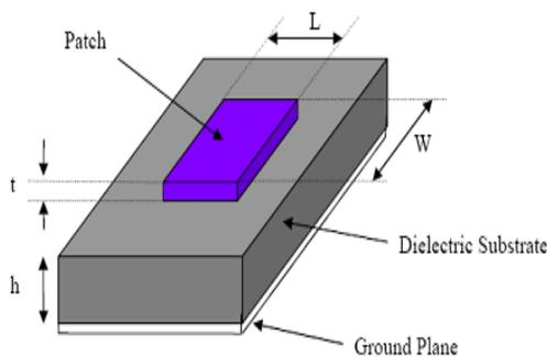
**Fig.1. Structure of Microstrip Patch antenna**
