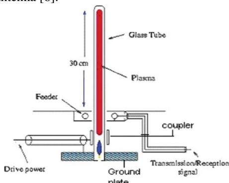
Fig. 4. A Schematic of the Experimental Setup of Plasma Applications
