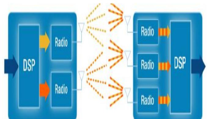
Fig. 5. Working of MIMO antenna
